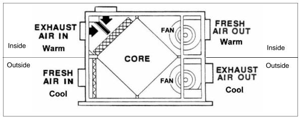
Air-to-air heat exchanger. Defrosting of the heat recovery core is critical to proper operation
