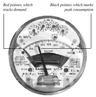
Conventional electrical demand meter. The red pointer records demand. As it moves up, it pushes the black pointer with it. When the red pointer falls back, the black pointer remains behind to mark peak consumption. Each month your meter reader records the reading on the black pointer.
