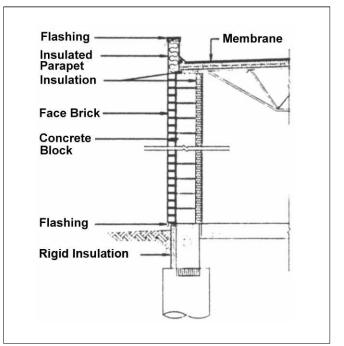
Typical brick and block wall construction
