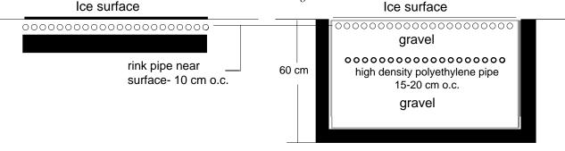
When the concrete floor needs to be replaced in 10 or 15 years, the thermal storage buffer can be installed.
