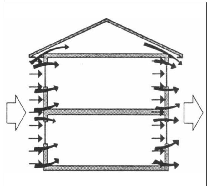
Usually the easiest element to convert to an air barrier will be the building's interior finish which can easily be caulked and repaired. Pay special attention to the details of the building, such as corners and joints with the ceiling and floor or partitions, to make sure there are no leaks.
