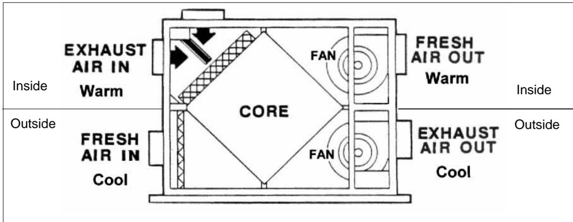
*Air-to-air heat exchanger. Defrosting of the heat recovery core is critical to proper operation*
