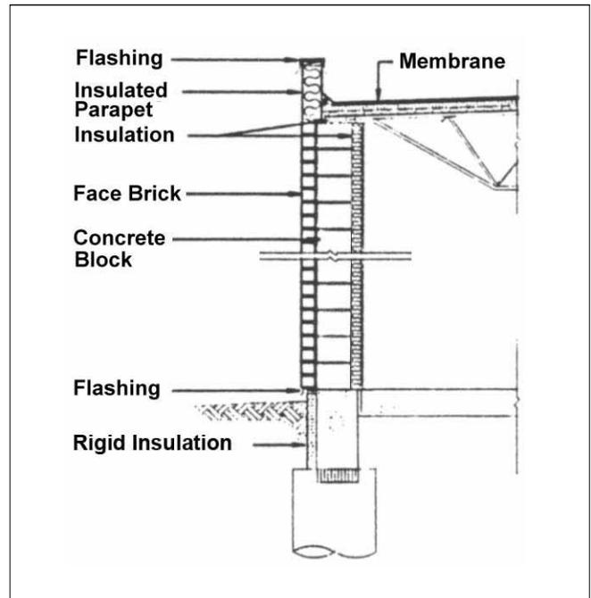
Typical brick and block wall construction
