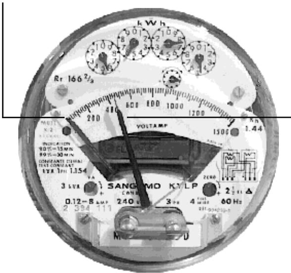
Conventional electrical demand meter. The red pointer records demand. As it moves up, it pushes the black pointer with it. When the red pointer falls back, the black pointer remains behind to mark peak consumption. Each month your meter reader records the reading on the black pointer.
