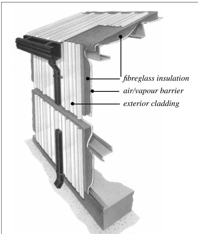
Energy efficient metal building. Standoffs between the interior metal liner and the exterior metal skin keep the insulation sandwiched in between from being compressed. The metal liner also serves as an air/vapour barrier.
