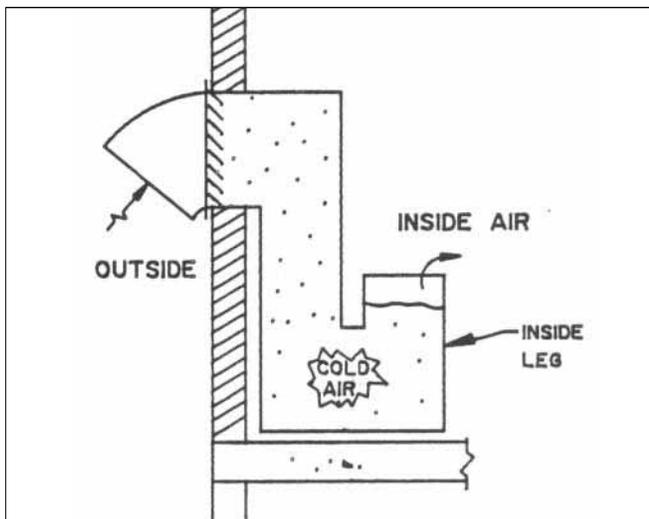
When the exhaust fans start the air is easily drawn through the ductwork.
